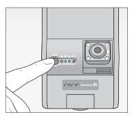
10. Turn on vehicle. Check that blue and green lights remain on after 5 minutes. If not, an error occurred. Press small, black button for 3 seconds. A beep confirms G-sensor calibration.
