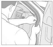
**7.** Tuck cable behind weather stripping, and push stripping in to secure it.
