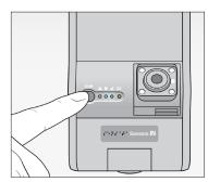
**10.** Turn on vehicle. Check that blue and green lights remain on after 5 minutes. If not, an error occurred. Press small, black button for 3 seconds. A beep confirms G-sensor calibration.
