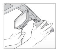
**5.** Remove backing. Press evenly to ensure the mounting bracket's adhesive is flush against the glass. Hold to window for 30 seconds.
