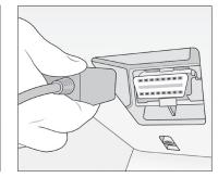
**9.** Plug end of OBDII adapter cable into vehicle's OBDII port. Ensure vehicle is on a flat surface for G-sensor and device calibration.
