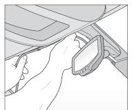
**6.** Remove adhesive and apply cable clips to windshield. Slide the bracket power cable into clips.
